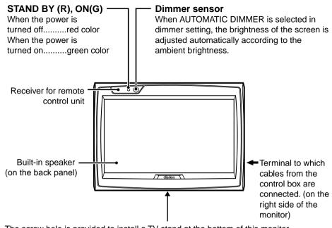
The screw hole is provided to install a TV stand at the bottom of this monitor. (1/4 inch unified screw thread, 4.5 mm of maximum length)
